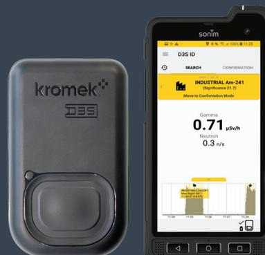
Complete radiation detection system for CBRN professionals that enables safe monitoring in high dose environments
